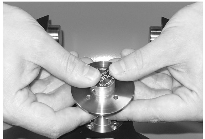
Figure 5. Removing the rotor
