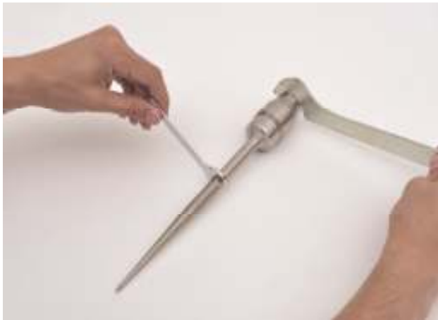
Replacement Tip Removal
