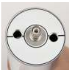
Feel for holes under the label and use a razor to expose both holes.
